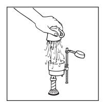
While holding a container over the uncapped VALVE to prevent splashing, turn water supply on and off a few times. Leave water supply off.
